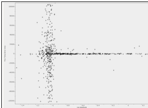
Figure 5: Logarithm of event amplitude (x axis) versus event match time (y axis) for the relaxed surface hypocenters. Surface events more than 1000 milliseconds from the y axis were classified as unverified.
