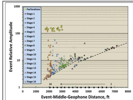
Figure 6: Logarithm of normalized event amplitude versus distance from the observation well for downhole events from stages 1-16. From Engelbrecht and Fuller, 2011.
