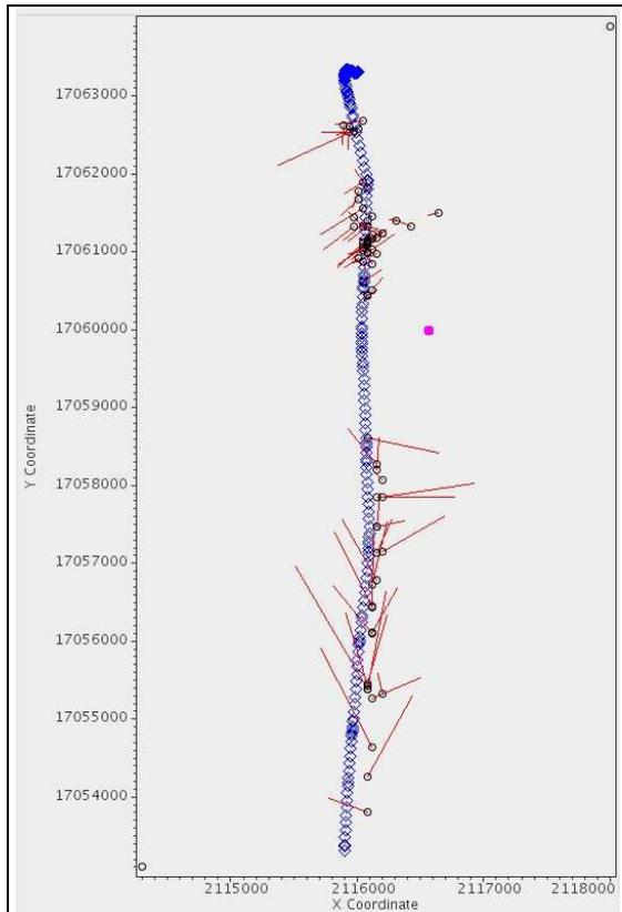
Figure 7: Location differences for matched events. The open circles represent the reported locations of the picks from the strict assessment of the surface data, the red line segments connect to the reported locations of the downhole data picks for matched events. All of the matched events were visually inspected, and in no more than 6 percent of the cases are there multiple events that are close enough in time to have caused a false match.
