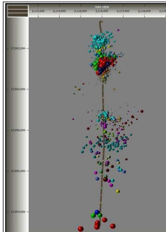
Figure 2: Map view of the hypocenters reported from the downhole data. The symbol sizes correspond to event amplitudes, and the colors correspond to stages. From Engelbrecht and Fuller, 2011.
