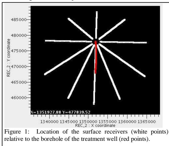
Figure 1: Location of the surface receivers (white points) relative to the borehole of the treatment well (red points).
